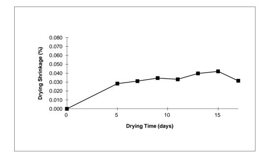
Note: Final linear drying shrinkage, S, is calculated by averaging the final length measurement at equilibrium with the previous two measurements for each specimen.
